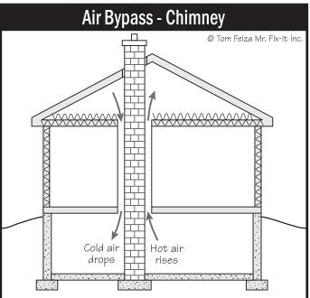
Masonry chimneys are always built with clearance to wood framing for fire safety. This area must be blocked with non-combustible material to prevent air movement.
