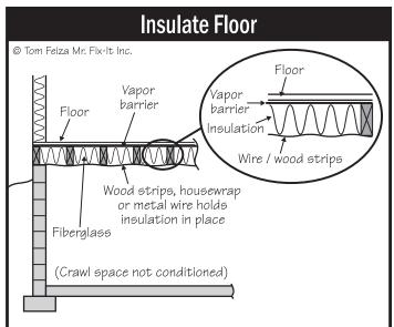
Floor insulation between the conditioned space and a non-conditioned crawl space is valuable. Note vapor barrier is on warm side.
