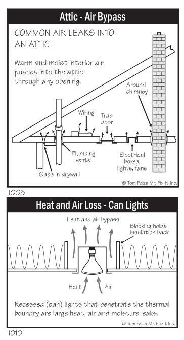
Want to find an air bypass into the attic? Lift the fiber insulation around the hatch door or near plumbing or electrical wiring. If you see darkened insulation, you have just found an air leak into the attic. The fiber insulation is black because it is filtering out dirt as air passes into the attic.
